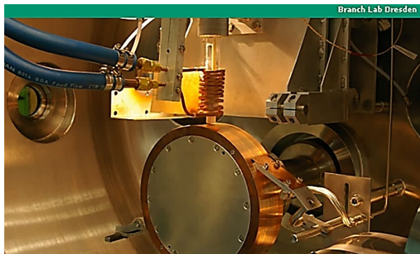
Fig. 2. The device used to produce ultra-fast hardened layers operates using the planar casting method.
